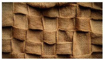
Coir based Biodegradable Geotextile
