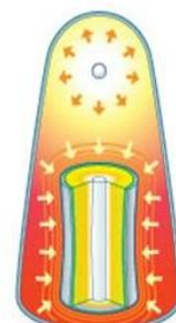
3. Foam, now a plasma, compresses secondary; fissionable "spark plug" ignites.
